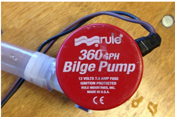
Figure 1. A 12 volt bilge pump works very well in a bucket wired to a solar module. This module produces 17 volts DC and moves water very handily when exposed to the sun.
