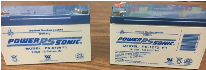
Figure 12. Two sealed solar batteries. The battery on left is rated at 6 volts, 12 amp-hours, and the battery on the right is rated at 12 volts, 7 amp-hours.
