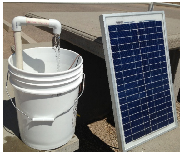
Figure 1. A 12 volt bilge pump works very well in a bucket wired to a solar module. This module produces 17 volts DC and moves water very handily when exposed to the sun.
