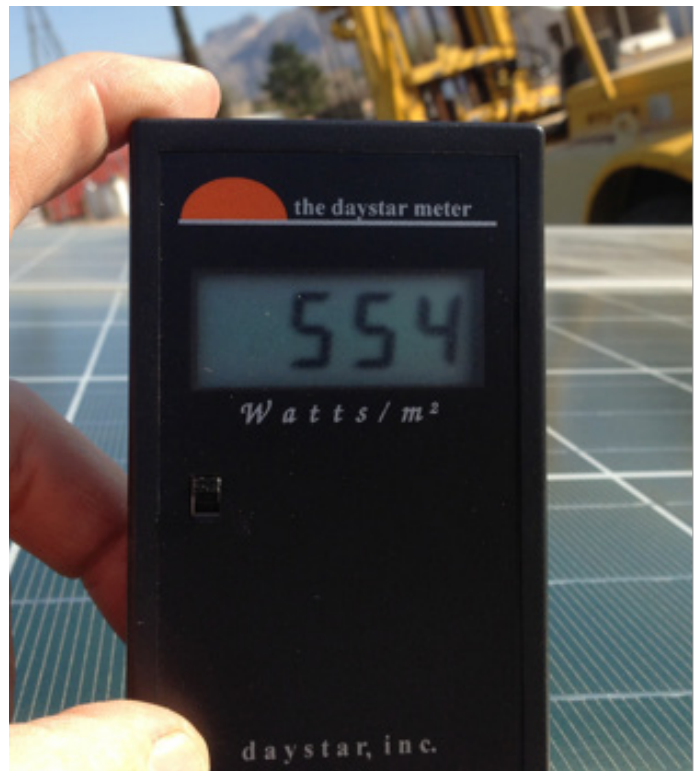
Figure 4. A solar irradiance meter (pyranometer) is used to measure the light intensity of the sun when the end of the meter is directed at the sun. Solar module power values are based on an irradiance level of 1,000 W/m 2 . Source: Author
