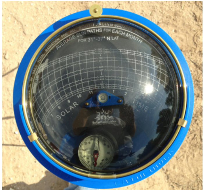
Figure 7. A Solar Pathfinder™ can determine where shading will come from surrounding a site and the amount of shading over the course of a year and at times of day from 6 AM to 6 PM. Source: Author
