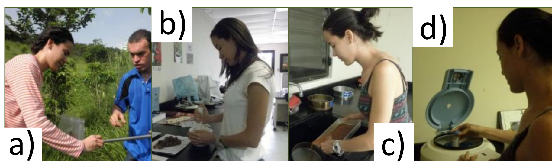
Figure 2. YSEG Scholar conducting the nematode sampling and processing: a) collecting soil samples at UPRU site; b) grinding soil samples; and extraction of nematodes using c) sieves and d) centrifuge.
