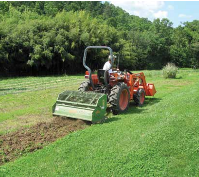
Mark Cain at Dripping Springs Garden uses a rotary spader for primary tillage. Photo by Heather Friedrich.
