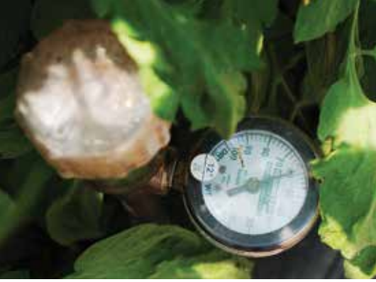
Tensiometers can be used to measure soil moisture and determine irrigation needs. Photo by Luke Freeman.
