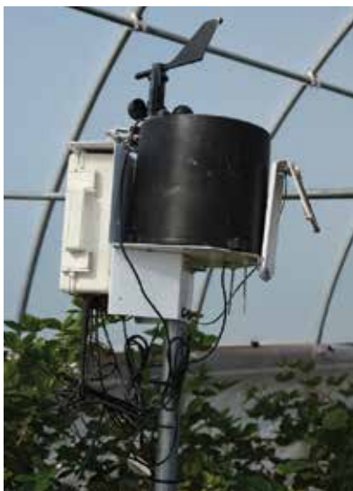
A weather station equipped with a rain bucket can be used to measure rainfall received. Photo by Luke Freeman.
