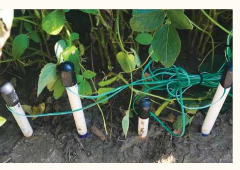
Soil moisture sensors that signal when to start and stop irrigation are installed in this soybean field at depths of 6, 12, 24 and 36 inches. Photo by Drew Gholson, Mississippi State University Extension
