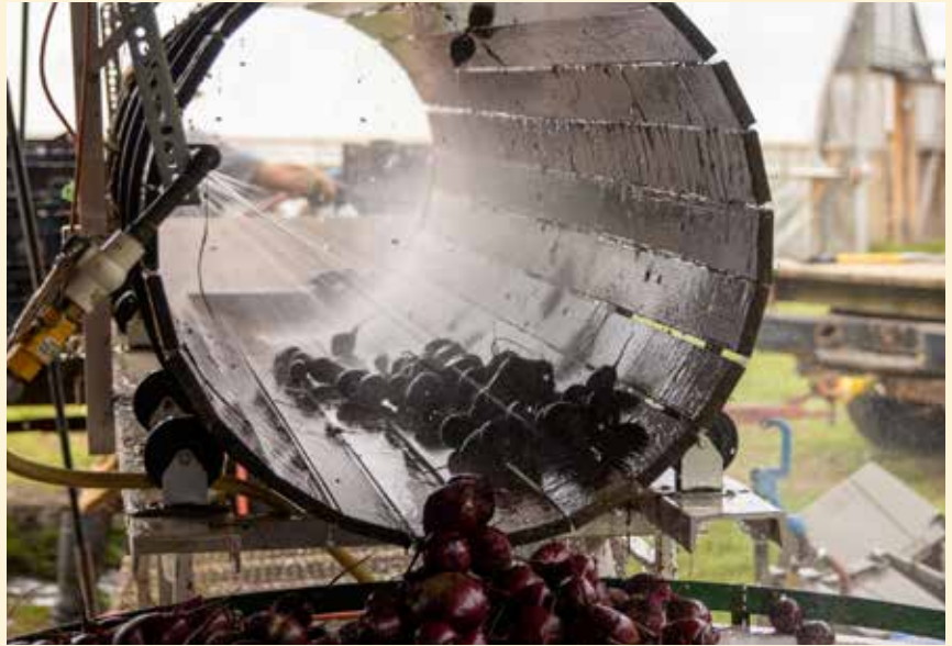
A barrel washer is used for rinsing beets. Photo by Andy Chamberlin, University of Vermont Extension
