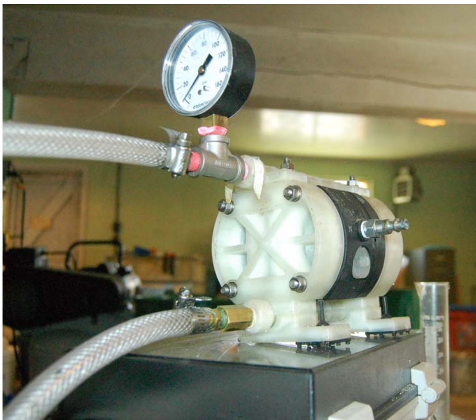
Figure 3: A small diaphragm pump.
