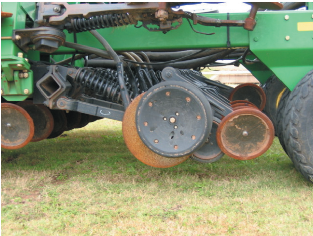
Figure 2. One of the most popular no-till drill designs uses a single disc opener that both slices through residue and opens the seed trench.
