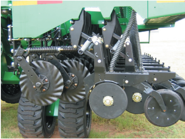
Figure 1. Some no-till drills, such as the one shown above, use a coulter that slices through residue and performs a small amount of tillage in front of the disc-opener.
