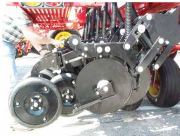
Figure 6. A Sunflower no-till drill with parallel linkage system.
