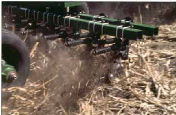
Figure 10. Tillage action of coulters on a no-till drill.
