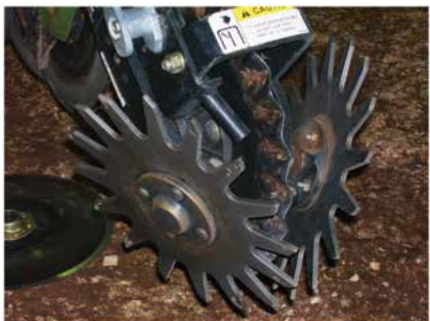
Figure 19. A combination coulter/row cleaner.
