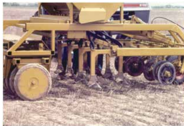
Figure 12. A Haybuster no-till hoe drill. Note the under frame clearance for residue flow.
