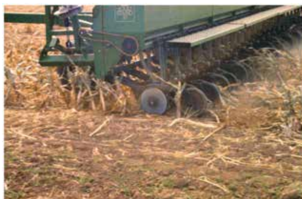
Figure 8. A Great Plains no-till drill with a swing arm linkage system.
