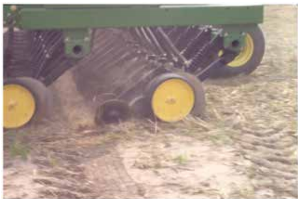
Figure 5. A single-disk opener operating in wheat stubble.
