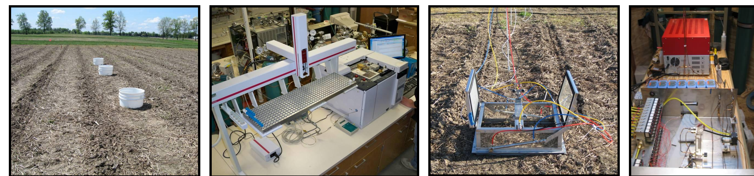
Figure 3. Static and automatic chambers sampling and analysis
