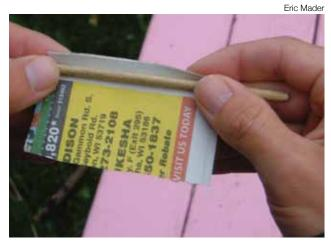
**Figure E.7** Paper being wrapped around a wooden dowel to make a paper tube liner.
