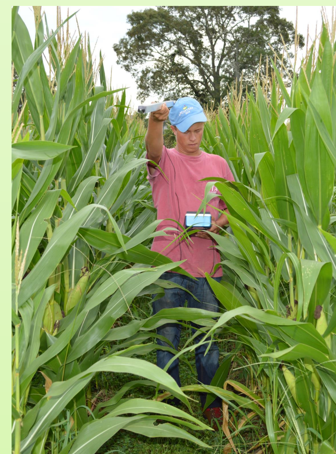
Figure 3: Measuring light interception (shading).
