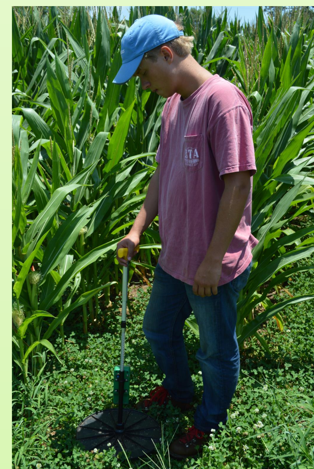
Figure 2 Using the RPM to measure clover mass
