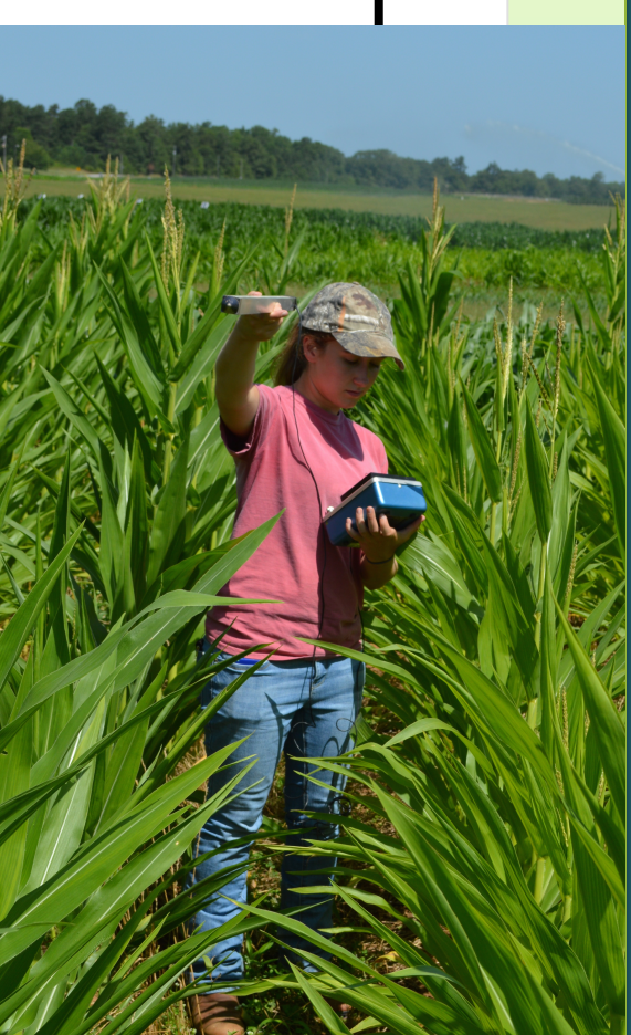
Figure 3: Measuring light interception.
