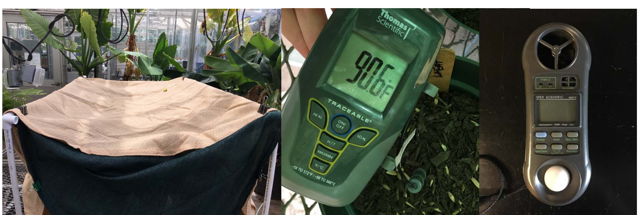
Images 5. The treatments were grown in greenhouse conditions under PVC with burlap covering. Images 6 & 7. Soil temperature was measured using a Thomas Scientific Traceable. Light flux and humidity were measured with a Sper Scientific 850070.
