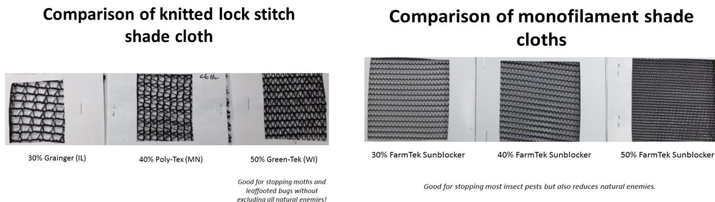
Fig. 1 shows the difference between knitted lock-stitch shade cloth with wide openings compared to monofilament shade cloths with narrow openings in Fig. 2.
