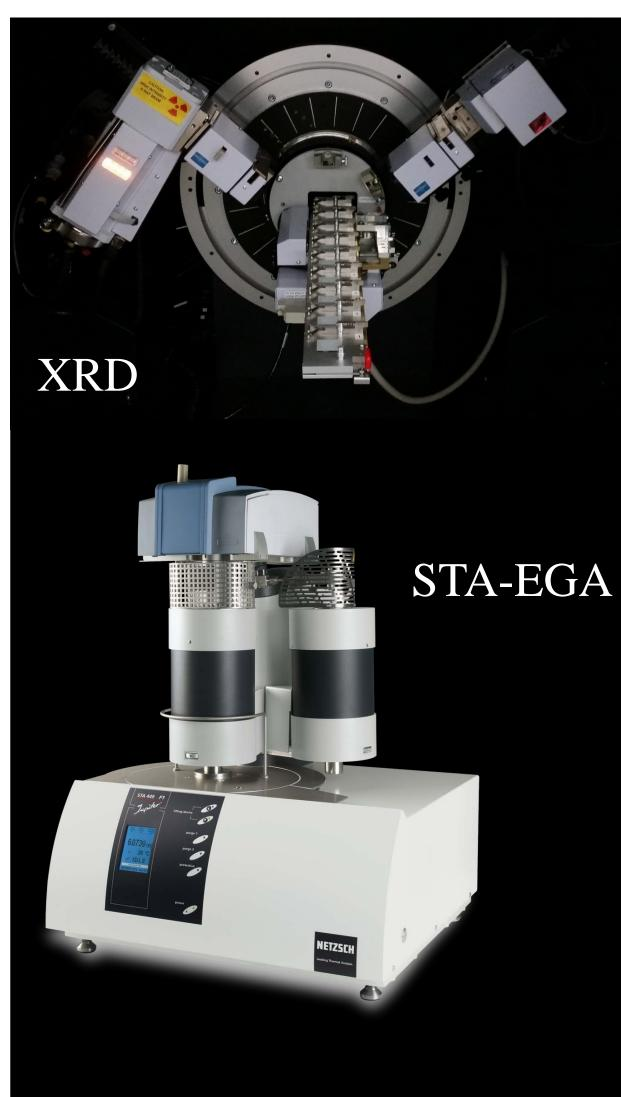
Analytical methods: Fertilizer collected from aerated-FBR was analyzed for mineral composition with X-ray diffraction (XRD; Bruker, D-8 advance). Thermal stability of the fertilizer product is evaluated using simultaneous thermal analysis with evolved gas analysis (STA-EGA; Netzsch, Perseus). Effluent composition for nutrient and pollutants removal is tested using colorimetry (DR-3900, Hach) and inductively coupled plasma optical emission spectrometry (ICP-OES).
