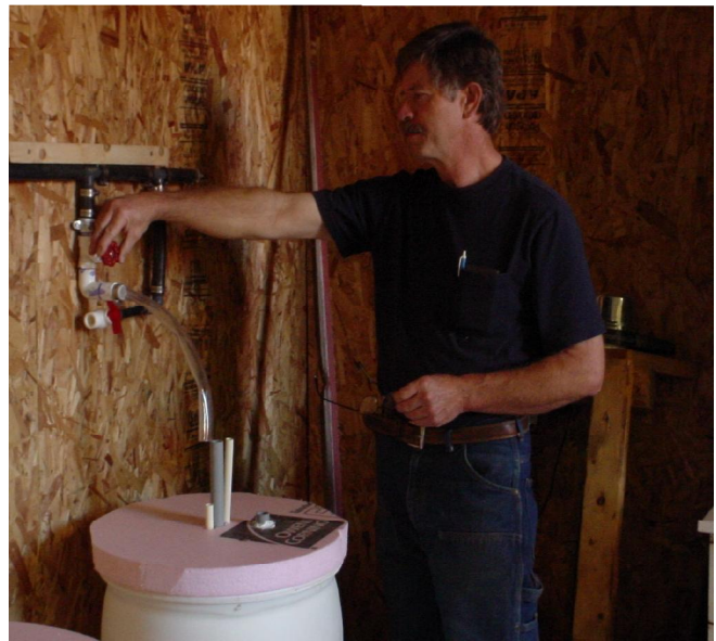
30-gallon insulated containers allow Eric Jellum to increase the number of treatments to evaluate various composting condition parameters more quickly than would be possible with larger bunkers. Projects such as this demonstrate composting for heat recovery (NCR-SARE project FNC05-562).
