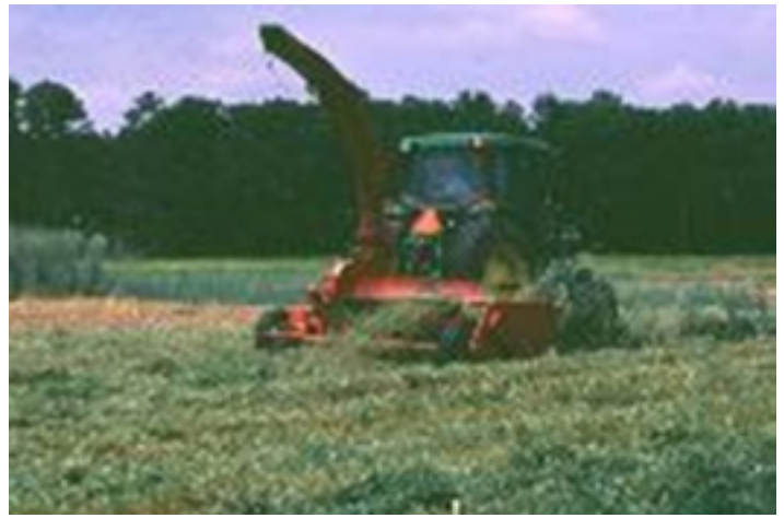
Figure 2. Flail chopper mowing a winter cover crop of annual hairy vetch and rye . Credits: D. Treadwell
