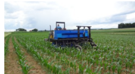
Figure 1. The Penn State Cover Crop Interseeder and Applicator. (Photo: Greg Roth)
