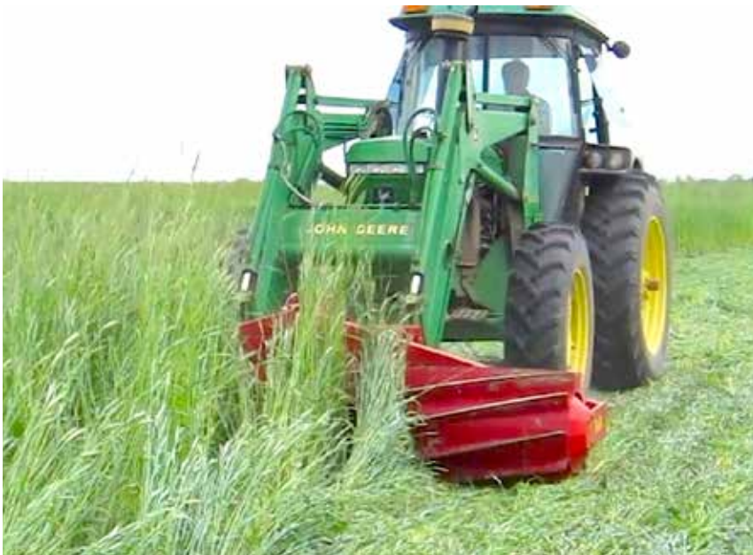
A roller crimper being used to terminate growth of cereal rye.
