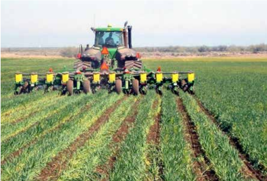
At top: Strip-till soybeans planted into corn residue. Photo courtesy of Jodi De-long-Hughes, University of Minnesota. At bottom: Planter configured to create narrow tilled strips while planting into cover crop residue. Photo courtesy of Paul Jasa, University of Nebraska.
