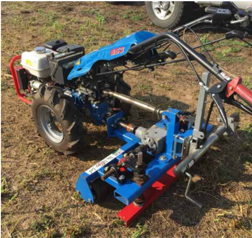
Example of a cover crop crimping attachment for a BCS walk-behind tractor.
