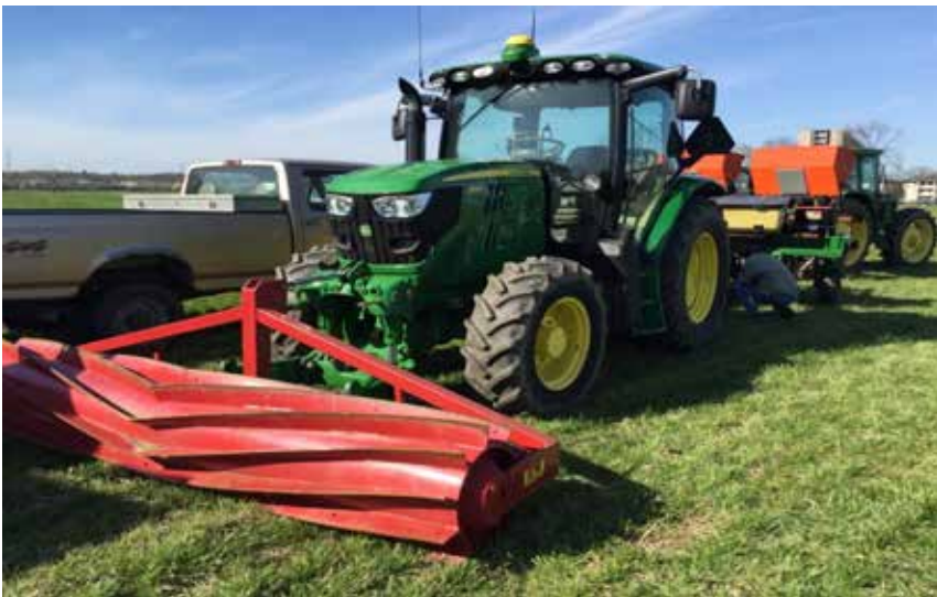
Example of a tractor set up with a front-mounted roller crimper and a row-crop planter attached to the rear of the tractor.
