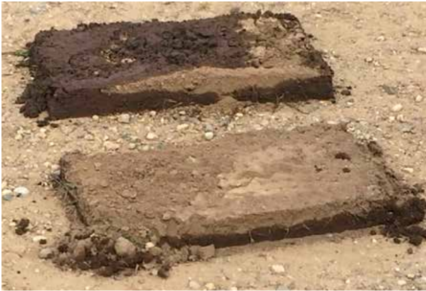
At top: A rainfall simulator, with tilled soil (second pan from left) showing most of the rainfall running off the soil into the front jar, while the cover-cropped soil allowed the rain to infiltrate into the soil and drain into the back jar underneath the soil tray. At bottom: the two trays of soil flipped over after an inch of simulated rain from an overhead sprinkler. The tilled soil in the foreground sealed shut after the sprinkler started running, preventing the simulated rainfall from soaking through, while the macropores in the no-till cover crop soil allowed the water to quickly soak into the soil.
