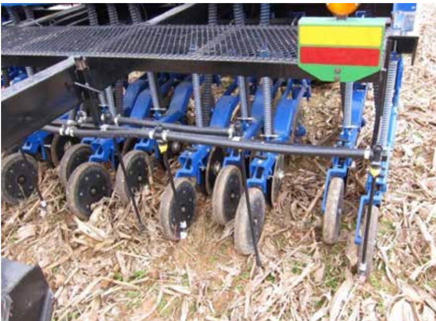
At top: A prototype high clearance drill for interseeding cover crops developed at Penn State University. At bottom: The rear of the drill, showing the skip row (blank area with no planter unit) for planting into existing corn with drop nozzles for herbicide and/or liquid fertilizer application.
