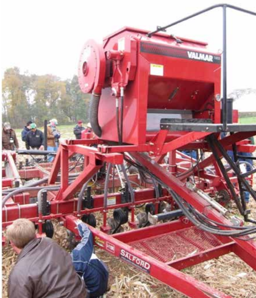
A Salford vertical tillage tool modified with an air seeder for cover crop planting.
