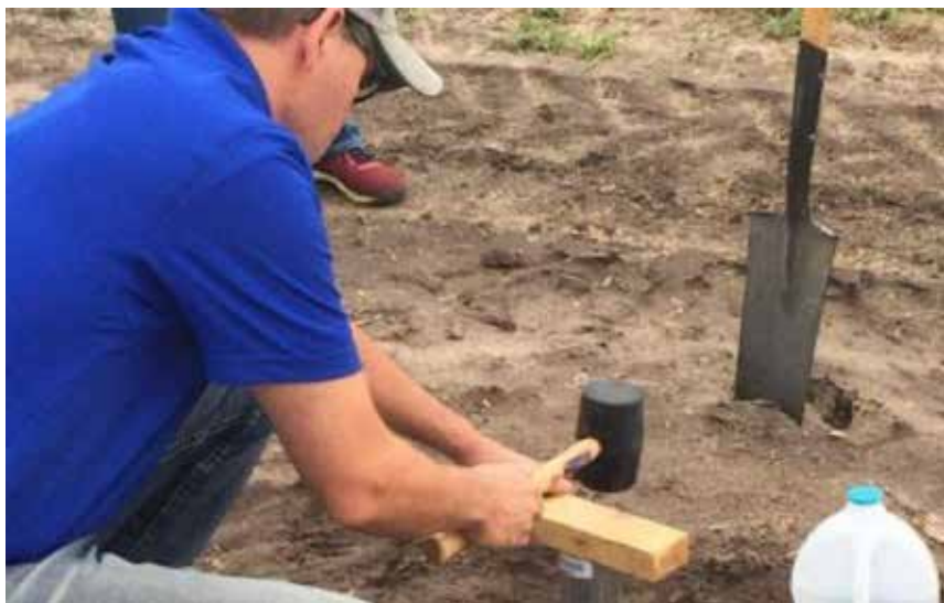
Using a bulk density ring to get an intact soil sample as part of soil health assessment. Photo courtesy of Rick Koelsch, University of Nebraska.
