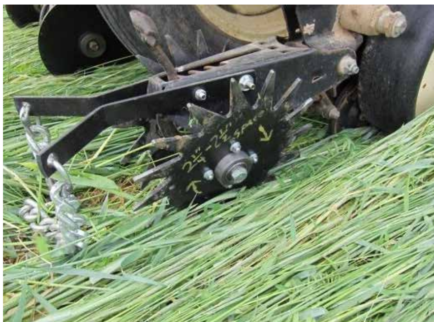
At top: The results of a roller crimper knocking down and terminating cereal rye. At bottom: spiked closing wheels being used to help close the seed furrow.
