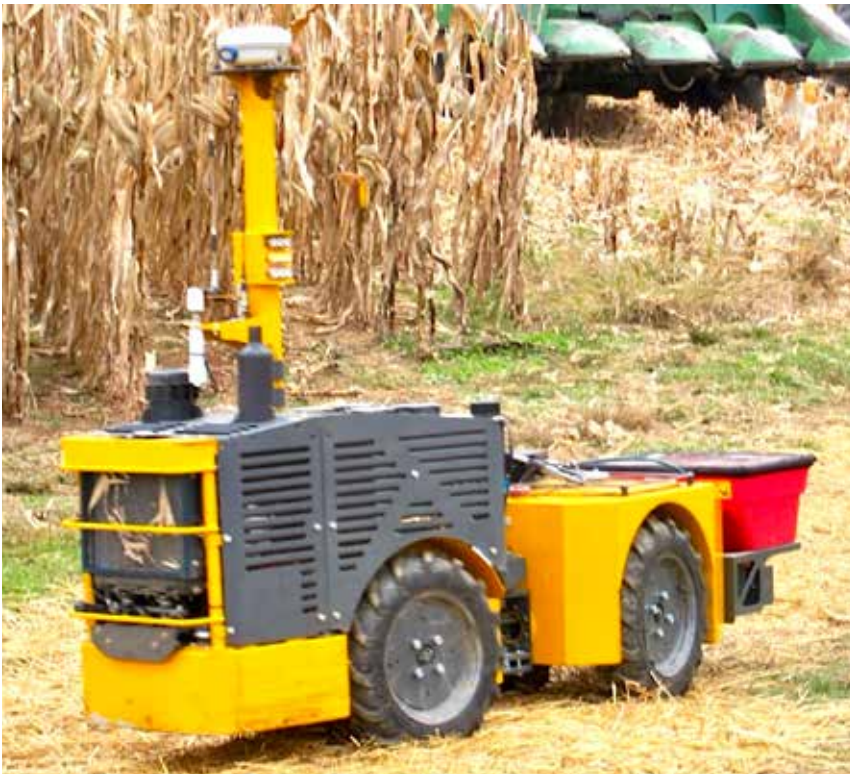
An early prototype of the Rowbot interrow diesel-powered unit. Newer models have tracks instead of wheels and can spread cover crops or fertilizer in an autonomous fashion between rows.
