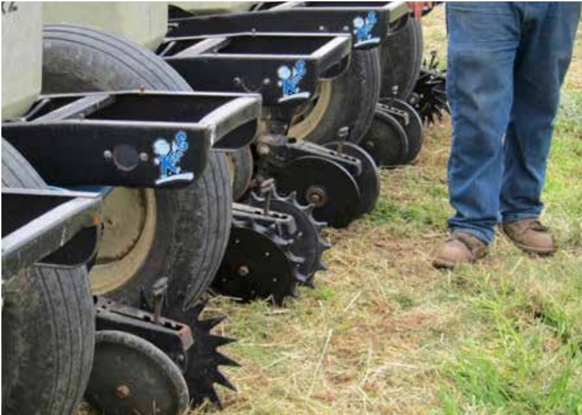
A University of Missouri planter temporarily modified with a variety of closing wheels to see what worked best while planting green. Farmers can benefit from trying a few different closing wheels to evaluate what works well for their soil and cover crop situation.
