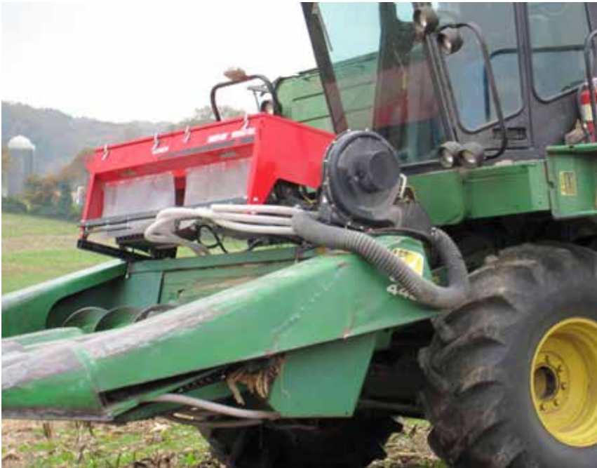
Gandy air seeder attached to corn head, with drop tubes that distribute seed under the corn head.
