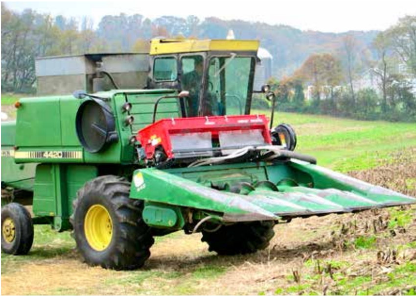
A combine modified with a Gandy air seeder that blows seed on ground underneath the corn head. Demonstration on Steve Groff's farm.
