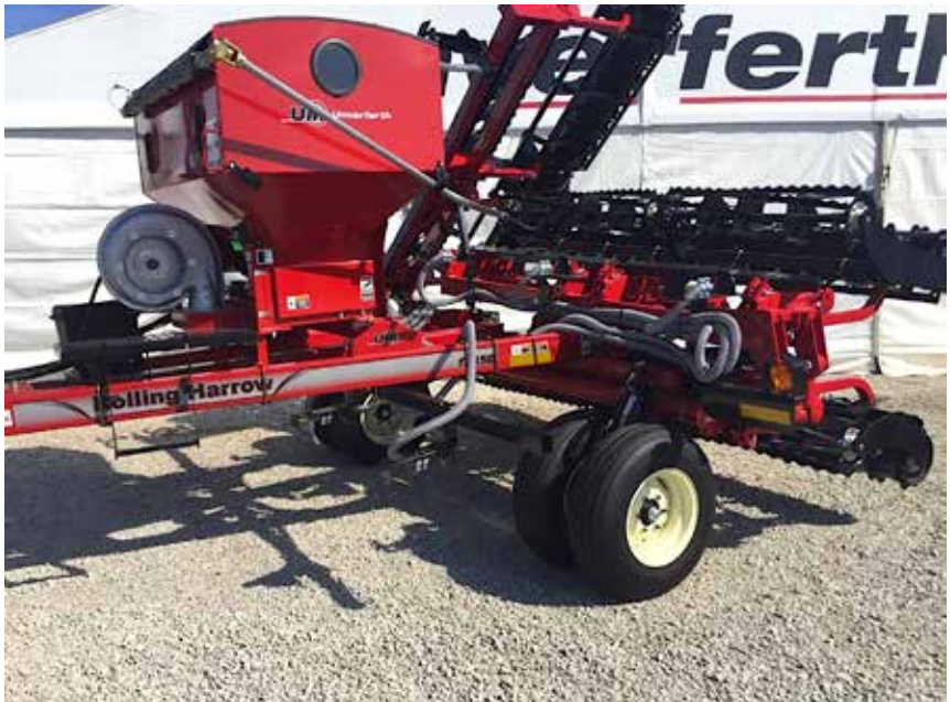
At top: Kuhn vertical tillage tool with optional cover crop air seeder. Several companies have similar options. At bottom: A rolling harrow set up with a cover crop air seeder.
