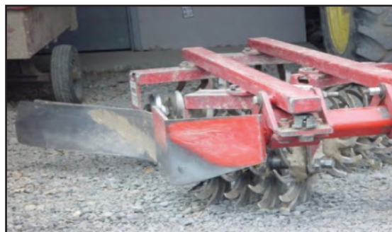
Figure 7: This Lilliston cultivator can be used for light tillage for weed control in the top few inches of soil as well as for incorporation of cover crop residues.
