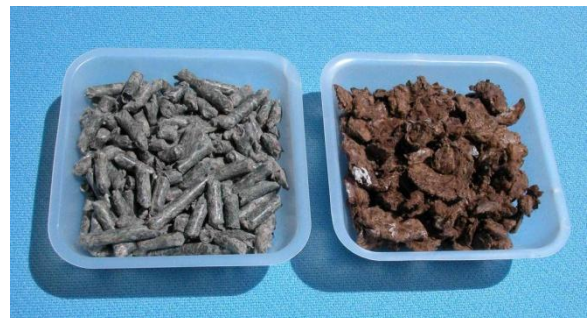
Figure 4. Examples of pelletized and processed and colored recycled newspaper that can be used as a mulch.
