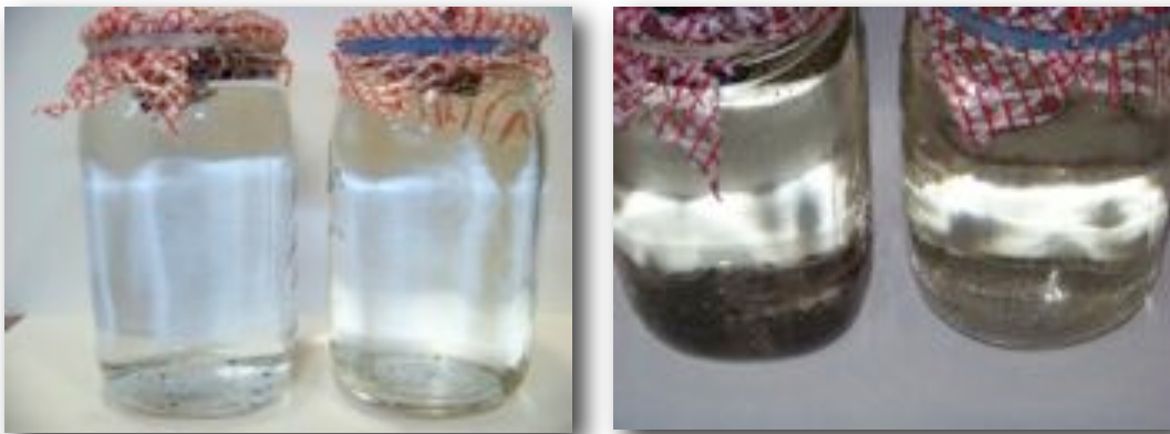
Poorly structured soil dissolves readily in demonstration jars, just like it does in field conditions leading to gully erosion.
