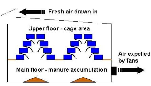
**Figure 1.** Schematic of a high-rise layer structure. Fans in the wall of the structure draw air out under negative pressure (suction). This pathway of air flow serves to vent ammonia and other gasses out of the structure, minimizing exposure of poultry.
