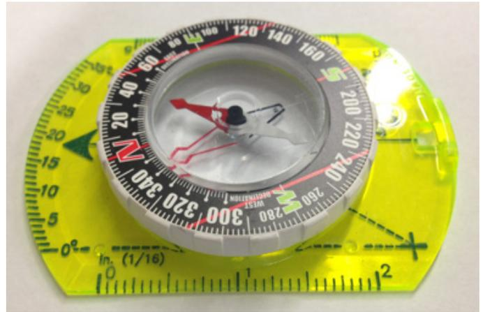
Figure 6. An azimuth compass is used to determine the best orientation for a PV array.
