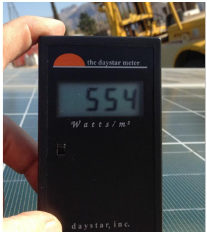
Figure 4. A solar irradiance meter (pyranometer) is used to measure the light intensity of the sun when the end of the meter is directed at the sun. Solar module power values are based on an irradiance level of 1,000 W/m<sup>2</sup>. Source: Author
