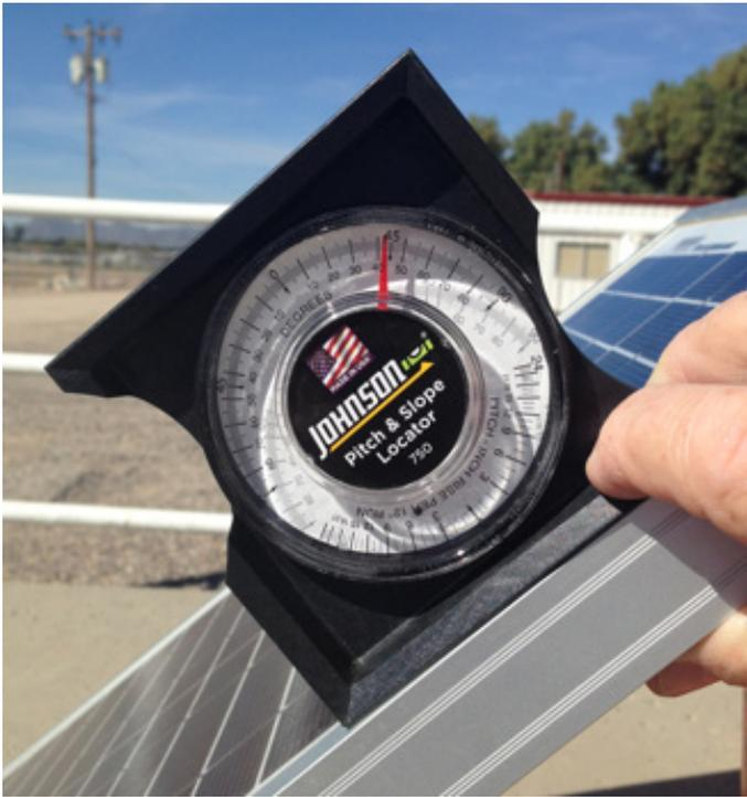
Figure 5. An inclinometer is set on the frame of the module and gives the tilt angle in degrees when the module is raised or lowered.
