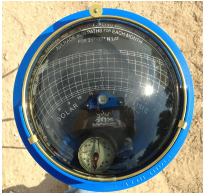
Figure 7. A Solar Pathfinder™ can determine where shading will come from surrounding a site and the amount of shading over the course of a year and at times of day from 6 AM to 6 PM.
