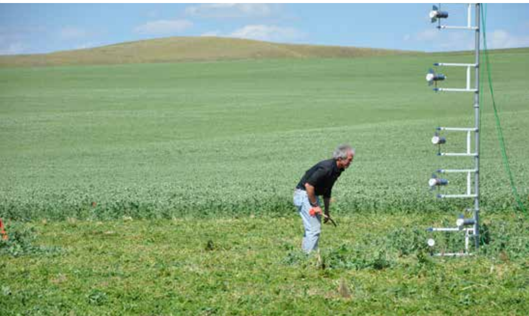
Montana State University scientist Rick Engel and his team used the integrated horizontal flux method to measure ammonia gas loss on a farm in Havre, Mont. They developed practical recommendations for how farmers can minimize atmospheric nutrient losses when fertilizing crops. Courtesy Rick Engel, Montana State University
