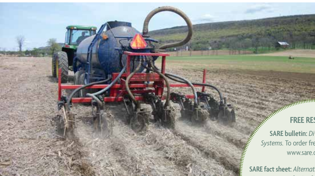
Penn State researchers have found that dairy farmers can save up to 70 pounds of nitrogen per acre by injecting manure instead of broadcasting it. Photo by Robert Meinen
