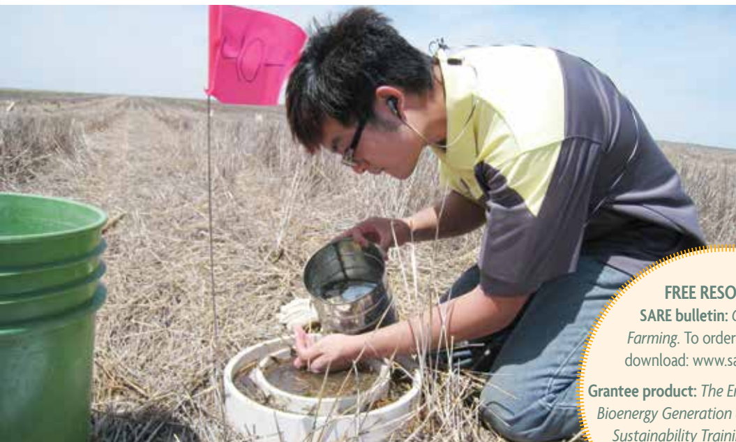
Kansas State University graduate student Yuxin He uses a double-ring infiltrometer to study how wheat straw residue affects water infiltration, part of KSU soil scientist Humberto Blanco's research on crop residue removal's impact on soil properties. Courtesy Kansas State University
