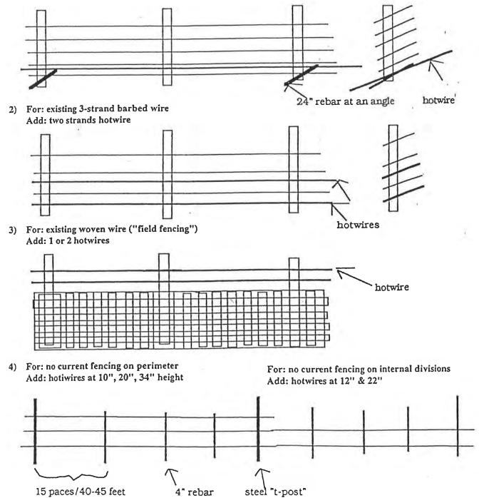
This fence works very well with aluminum low-tensile wire, but probably wouldn't with high-tensile, unless it was in a very straight line!
