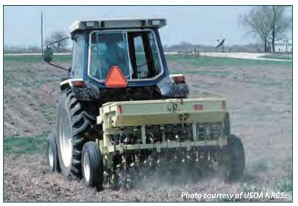
No-till grass seeders ensure proper seed placement and result in better germination.
