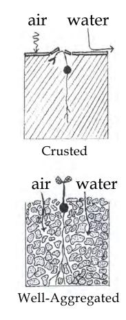
Figure 3. Effects of aggregation on water and air entry into the soil. Derived from Land Stewardship Project Monitoring Toolbox (15).
