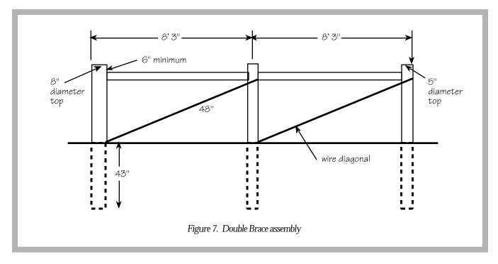
corner posts leaning back from the direction of the fence approximately five degrees. Brace wire should pull in the opposite direction than the fence is pulling.
