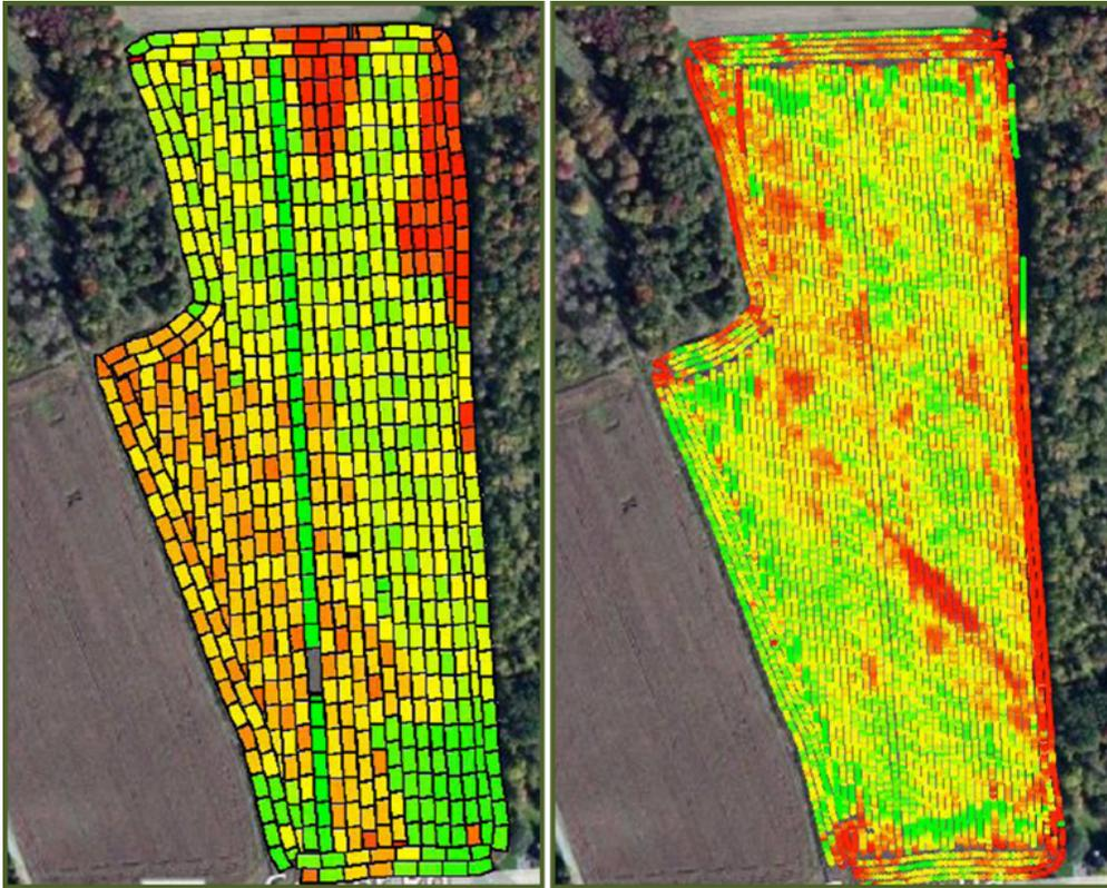
MAPPING TRIAL RESULTS. Top & Bottom (left): N application maps for Trials 48-50 and 38 & 39 respectively, retrieved from calibrated anhydrous sidedresser - the green strip indicates the high rate grower-N strip, and the grey rectangle indicates a zero-N section (data not discussed here). Top & Bottom (right): Yield maps retrieved from calibrated yield monitor, with no visually apparent yield increase with higher Grower-N rate in all trials.
