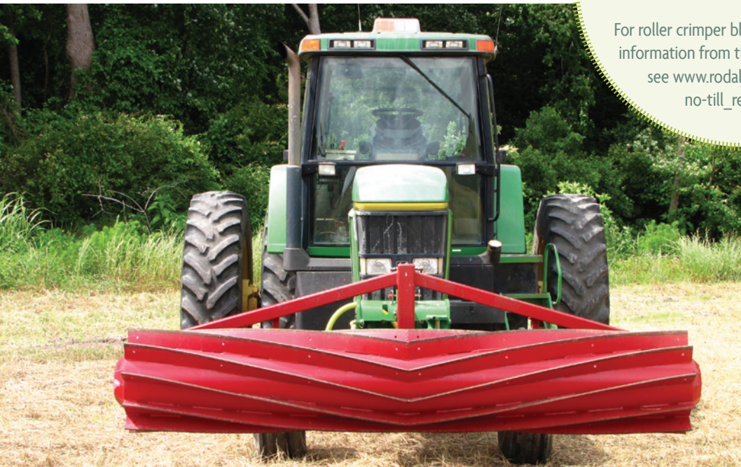
Roller crimpers, which roll down and crimp cover crops to establish a thick mulch, are being used by researchers around the country to demonstrate the tool's effectiveness in organic no-till systems. This roller crimper is at the Center for Environmental Farming Systems in Goldsboro, N.C. Photo by Andy Ziemiński, SARE Outreach
