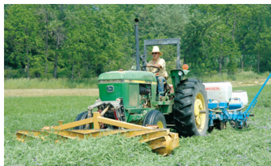
Jeff Moyer, director of farm operations at the Rodale Institute in Kutztown, Penn., uses a front-mounted roller to kill a hairy vetch cover crop, while a no-till planter drops seed corn behind the tractor. Photo by Matthew Ryan for the Rodale Institute
