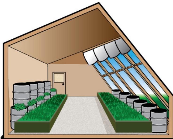
**Figure 16.** A typical passive solar greenhouse has well-insulated opaque surfaces, a glazed south wall pitched at an angle equal to the latitude, and water-filled barrels to collect heat.
