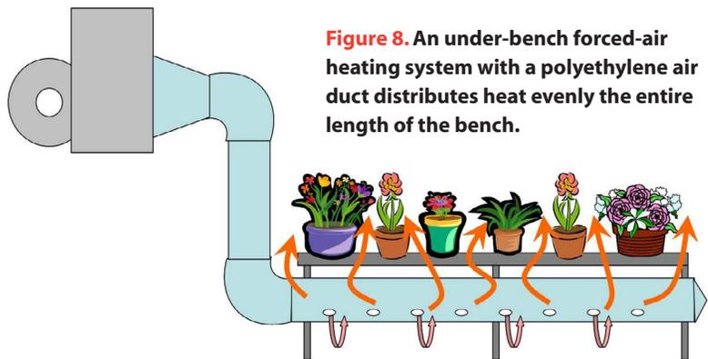
**Figure 8. An under-bench forced-air heating system with a polyethylene air duct distributes heat evenly the entire length of the bench.**
