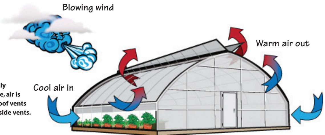
**Figure 13.** In a naturally ventilated greenhouse, air is sucked out through roof vents and flows in through side vents.
