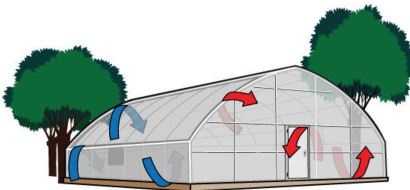
**Figure 1.** Greenhouse heat loss and gain pathways.
