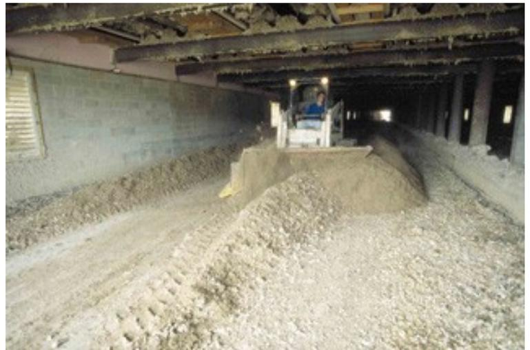
**Photo A.** A Brown Bear 24C compost turner [2] fitted to a skid-steer drive unit turns compost inside a high-rise layer structure.
