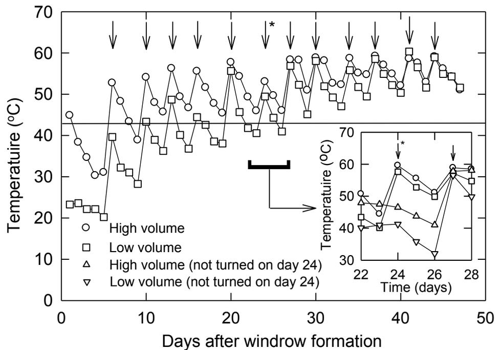
**Figure 2.** Daily compost temperatures measured during a seven-week in-house cycle. The treatments consisted of high and low initial volumes of composting material. Arrows indicate when compost was turned. The horizontal line represents the lethal limit for fly larvae (43 °C = approximately 110 °F). The \* indicates when certain replications of the treatments were not turned on day 24. Data from Miner et al. (2001) [5].
