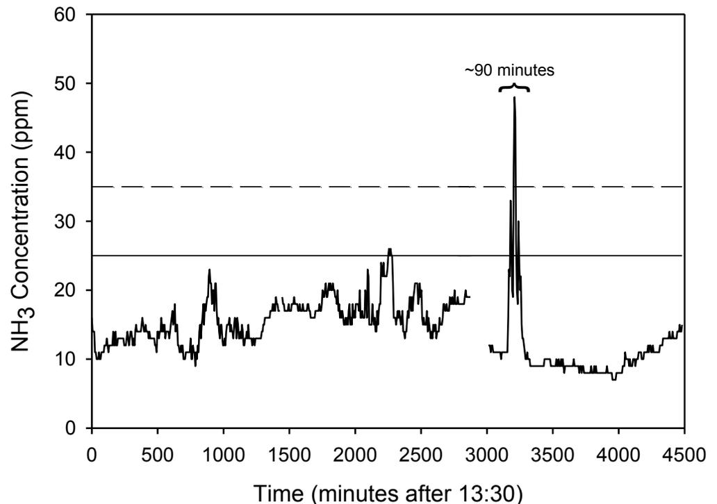
**Figure 3.** Ammonia concentrations over time in the manure storage area of a high-rise layer structure during in-house composting. The peak concentration occurred during a compost turning event. The — line indicates the 8 hour human health exposure limit. The - - line indicates the 10 minute human health exposure limit. Data are from Koenig et al. (in press) [9].
