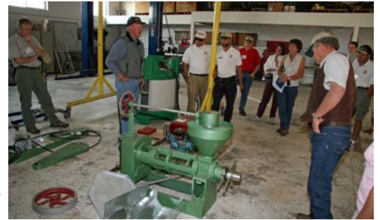
Bill Wright explains his new oilseed press from which he plans to make biodiesel from his oilseed crops that include sunflowers and camelina.
