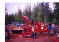
Chipping timber from slash piles.
