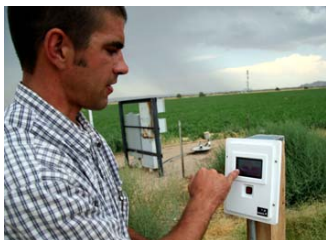
Grant Poole checks soil moisture levels through in-field monitors.
