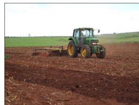
A harrow incorporates cover crop seed at a demonstration site.
