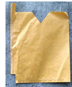
This wax-coated bag allows 46% light transmission.
