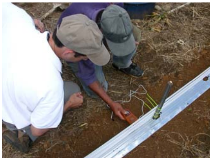
Aluminum building studs were bent flat along the ground under the electric tape
